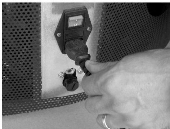
Figure 17 – Disconnect the stove from the electrical mains
