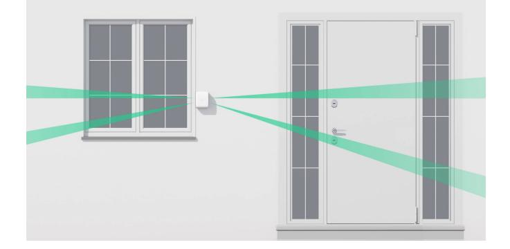
If one side of the detector is used to protect a door, and the other to protect a window, the detector is installed at the height of **0.5 to 0.6 meters from the window sill**. If the detector is placed close to a window, the Near area detection option should be enabled (the **Near area detection** switch on the back of the detector). The option reduces the blind spot near the detector.
