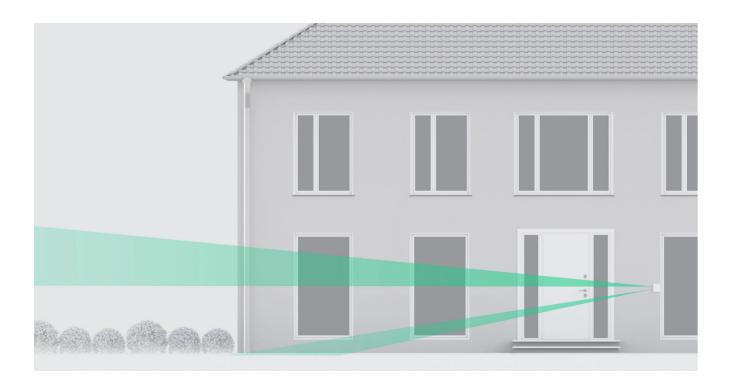
DualCurtain Outdoor includes two opposing curtain motion detectors. The detection distance is adjusted separately for each side with the **Detection Distance** scrollbars on the back of the detector.
