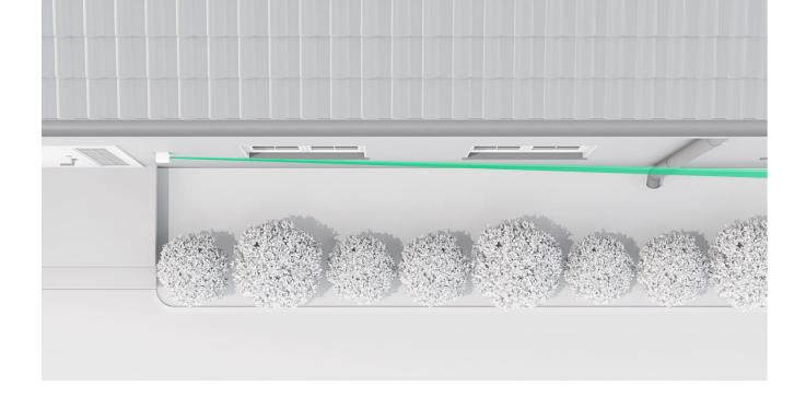
If appropriate, turn on **Near area detection** (**Near area detection** scrollbar) for the desired side. The mode allows the detector sensors to detect motion when an attempt is made to break in at the very body of the device, reducing the blind spot.
