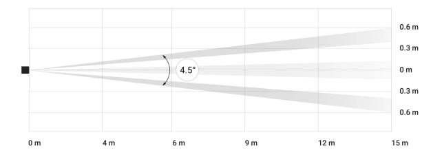
Horizontal viewing angle of the detector
