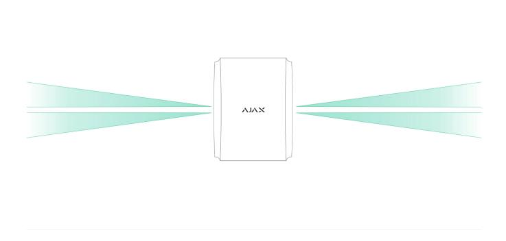
The detection distance for each side can be adjusted independently, allowing you to set the detection zone precisely and avoid false alarms caused by bushes, trees, or other objects.
