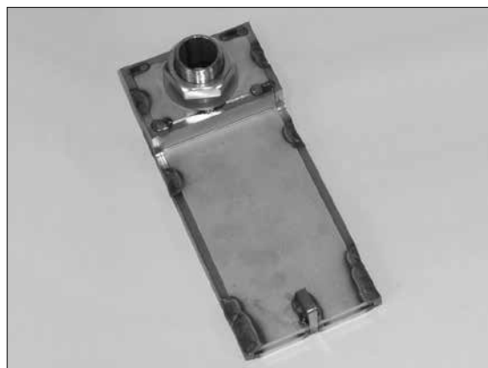
Pneumatic cleaning duct
