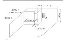
The national rules on installing electrical equipment in the bathroom must be scrupulously respected. The electric towel rail must be always installed outside zone 1 and 2.
