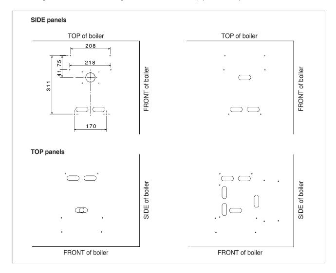
Once you have identified the right holes for the type of installation required, proceed as follows:
