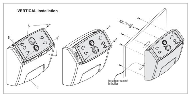
Before you can install the control panel on a boiler side panel, proceed as follows:
