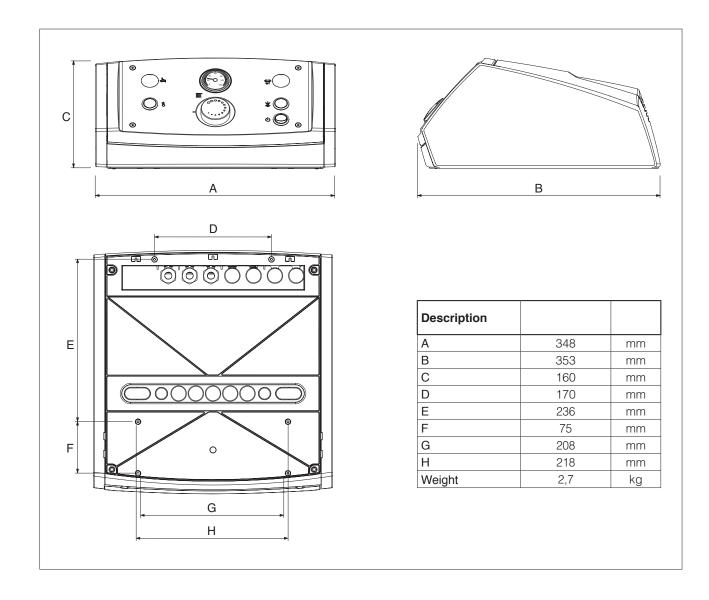
**RIELLOtech PRIME** control panels can be installed either on the top of the boiler or on one of its side panels. Before commencing installation, check the arrangement of the holes on the top panel or side panel of the boiler.
