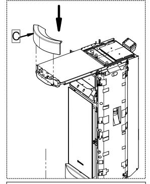
3 - Remove the tray and insert the upper majolica (C) on the teeth provided. Slightly bend the teeth so as to firmly secure the majolica to the body.
