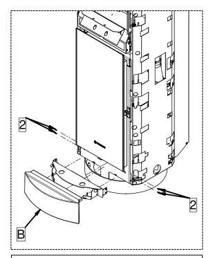
2 - Undo the 4 screws (2) and remove the majolica support bracket. Insert the lower majolica (B) on the bracket that you have just removed. Lastly fasten the bracket with the majolica using the 4 screws (2) just removed.
