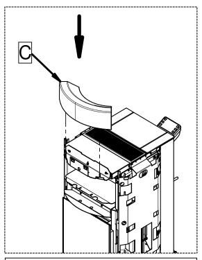
4 - Insert the upper majolica (C) on the teeth provided. Slightly bend the teeth so as to firmly secure the majolica to the body.
