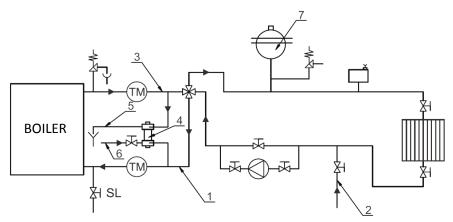
Figure 7 a – Scheme of closed central heating system with built in 4-way valve
