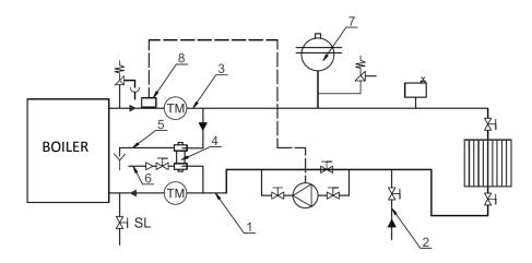
Figure 7 b – Scheme of closed central heating system with built leaning pipe thermostat
