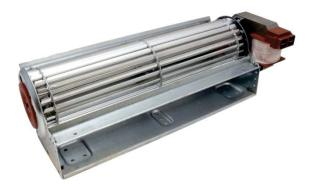
They have the function of removing heat from the warm surfaces of the stove and using the directional air to pass it over to the room. Its work can define a control unit in a way that automatically increases the speed of rotation in relation to the achieved temperature of the stove or that the user sets the fixed speed of rotation.
