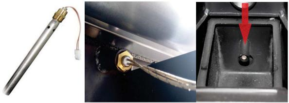
The heater is a device by which the incineration of the pellet or the first pellet dose in the burner is carried out. In all stoves and boilers, in addition to some industrial ones, identical 250W heaters are installed. They work at 230V AC. They are installed in the foreseen tube for which the end is in the bottom of the burner.
