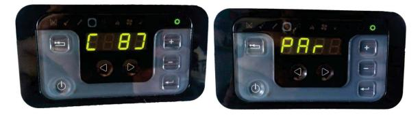
Clicking again ENTER will show the zero parameter parameter P000, the (+) and (-) keys are selected which parameter we want from P000 to P0105. After that, pressing ENTER will show the value of the parameter, which we increase or decrease with the (+) and (-) keys. After the correct value is set, pressing the ENTER key will save the parameter value.
