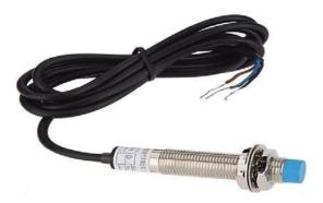
An inductive position sensor is a contactless sensor that has the ability to detect metal near the sensing head (about 2mm / max 4mm in front of the head surface). It is only installed in smart boilers and is an integral part of the mechanism of the mechanism with "self-cleaning burners". With it, the control unit counts how many times the burner executed the cycle of discharging the burner (factory 3 times) for one cleaning.
