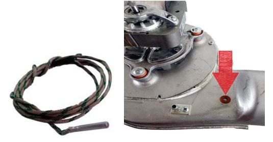
The sensor is intended for reading the temperature of the exhaust gases. The end of the sensor with the metal shield is placed in the required position on the exhaust fan housing as in the picture above. In the event that the fan is mounted on an adequate flange (in some versions of the boilers), the sensor is placed in the provided hole on the flange, it is necessary to ensure sealing between the sensor and the flange with a high temperature resistant silicone.
