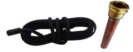
NTC is a negative temperature coefficient resistor which is used to measure the temperature of the liquid in the boiler. It is inserted into copper tubes in the form of a tube in such a way that the end of the sensor
