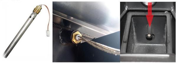
The heater is a device by which the incineration of the pellet or the first pellet dose in the burner is carried out. In all stoves and boilers, in addition to some industrial ones, identical 250W heaters are installed. They work at 230V AC. They are installed in the foreseen tube for which the end is in the bottom of the burner.
