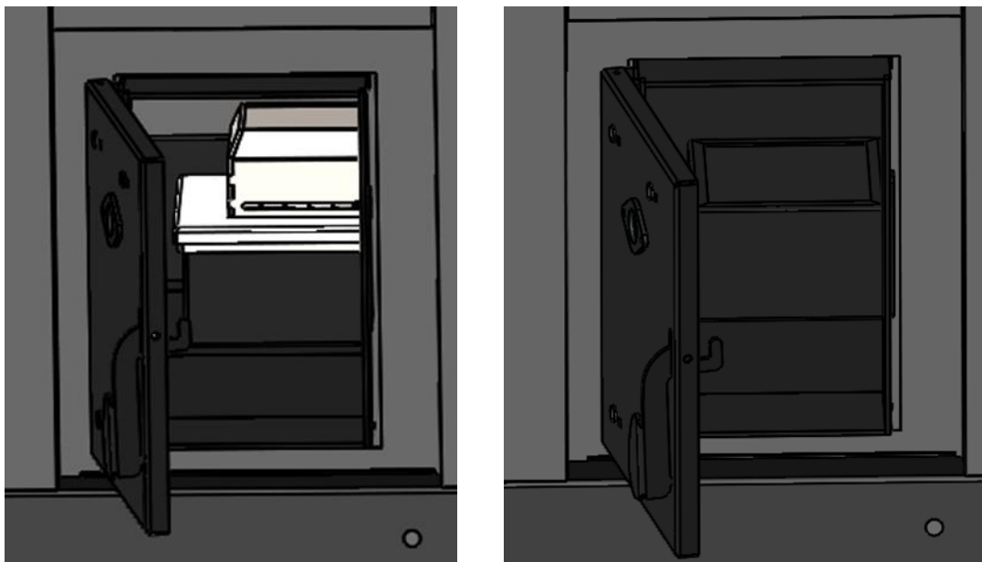
Figures 21 i 22. Cleaning of burner housing by vacuuming
