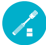
Torque wrench 10 - 30 Nm with socket for WS 13
