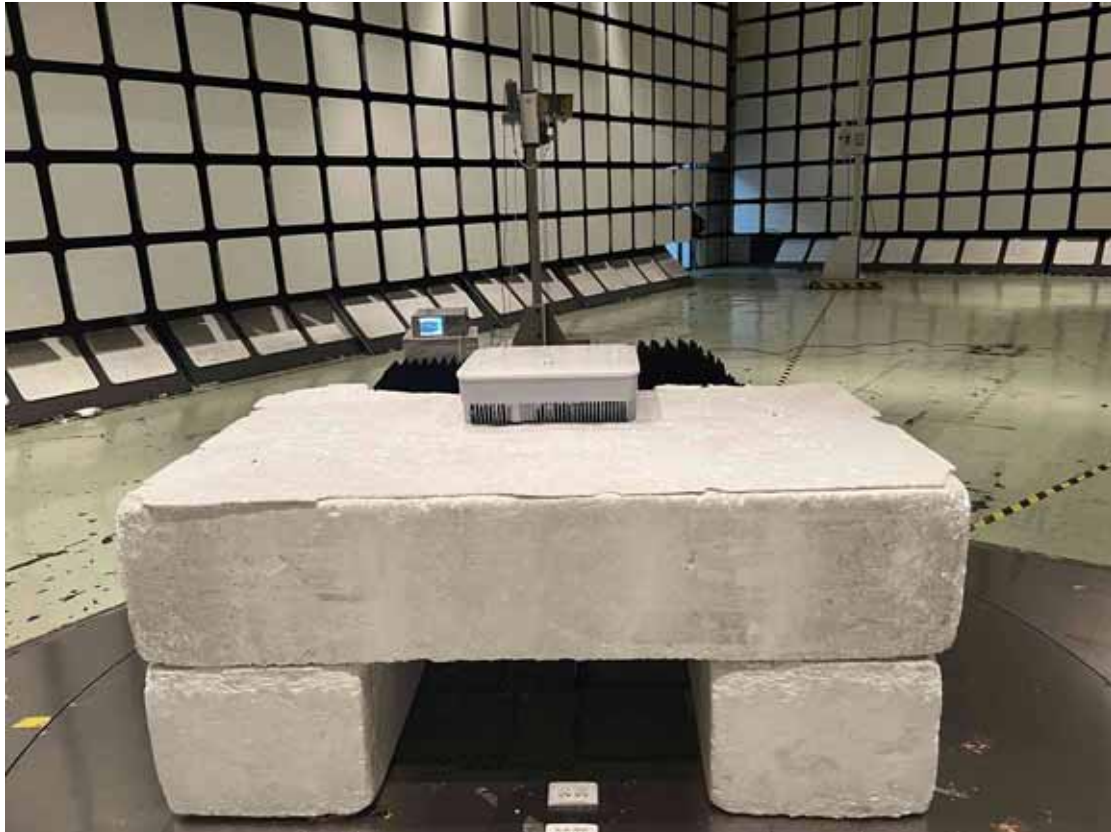
Front View of Radiated Disturbance Measurement
