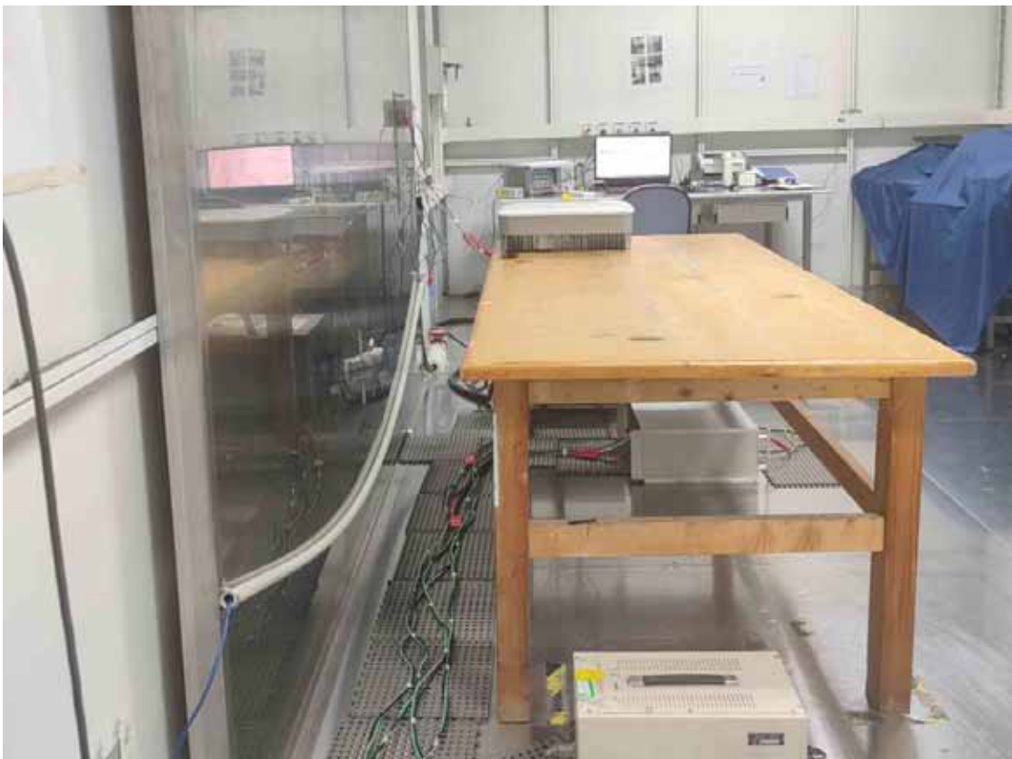
Front View of Conducted Measurement (DC Mains Port)
