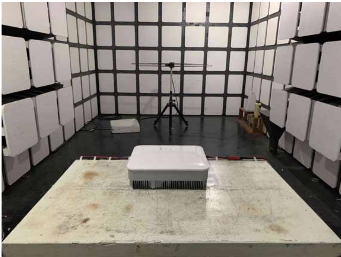
Front View of R/S Test (80MHz~1GHz)
