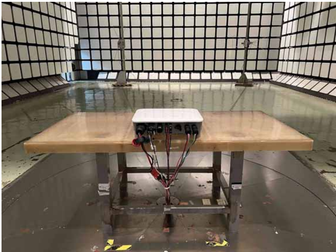
Back View of Radiated Disturbance Measurement
