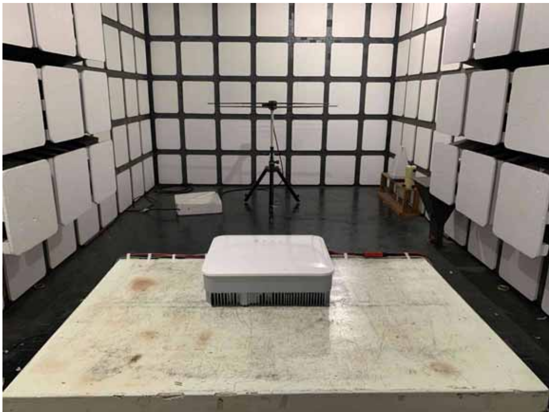
Front View of R/S Test (80MHz~1GHz)
