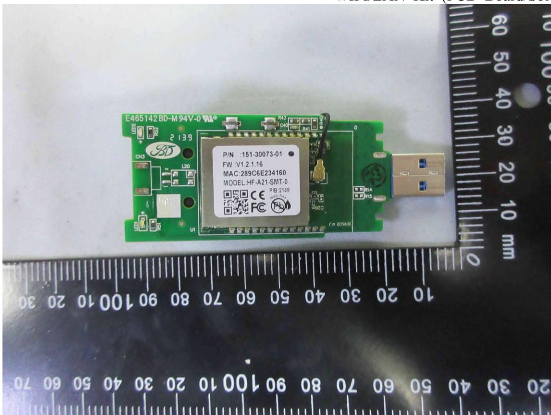
Figure 28 WIFI/LAN Kit (PCB Board/Solder Side)
