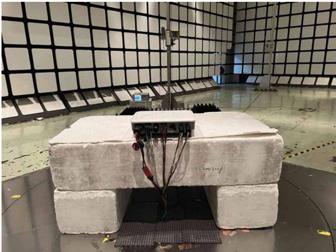
Back View of Radiated Disturbance Measurement
