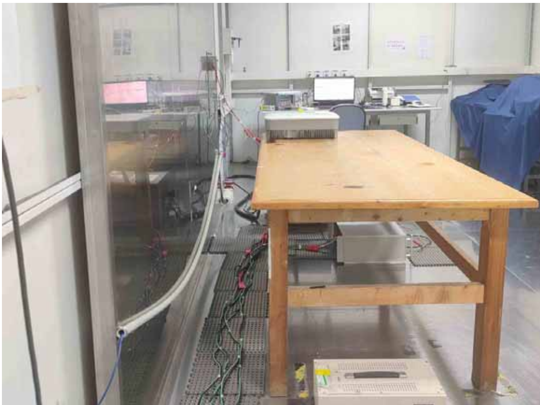
Front View of Conducted Measurement (Telecommunication Port)
