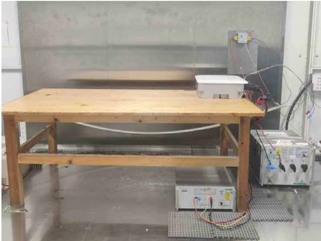
Front View of Conducted Measurement (Telecommunication Port)
