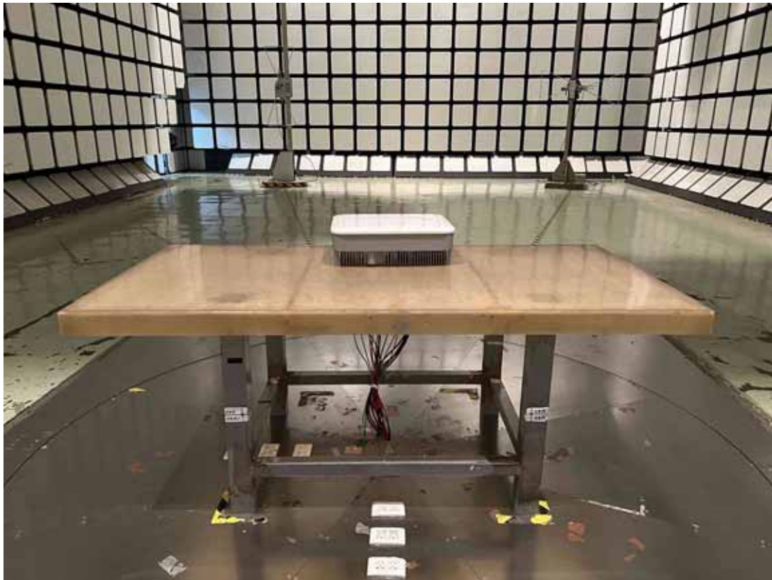
Front View of Radiated Disturbance Measurement
