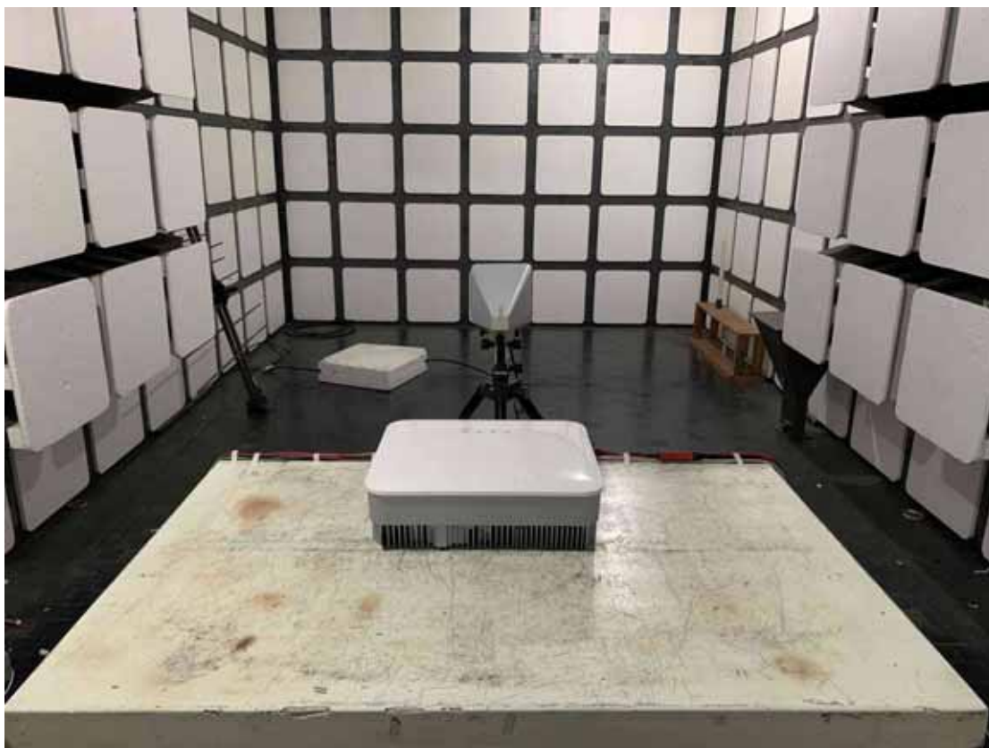
Front View of R/S Test (Above 1GHz)
