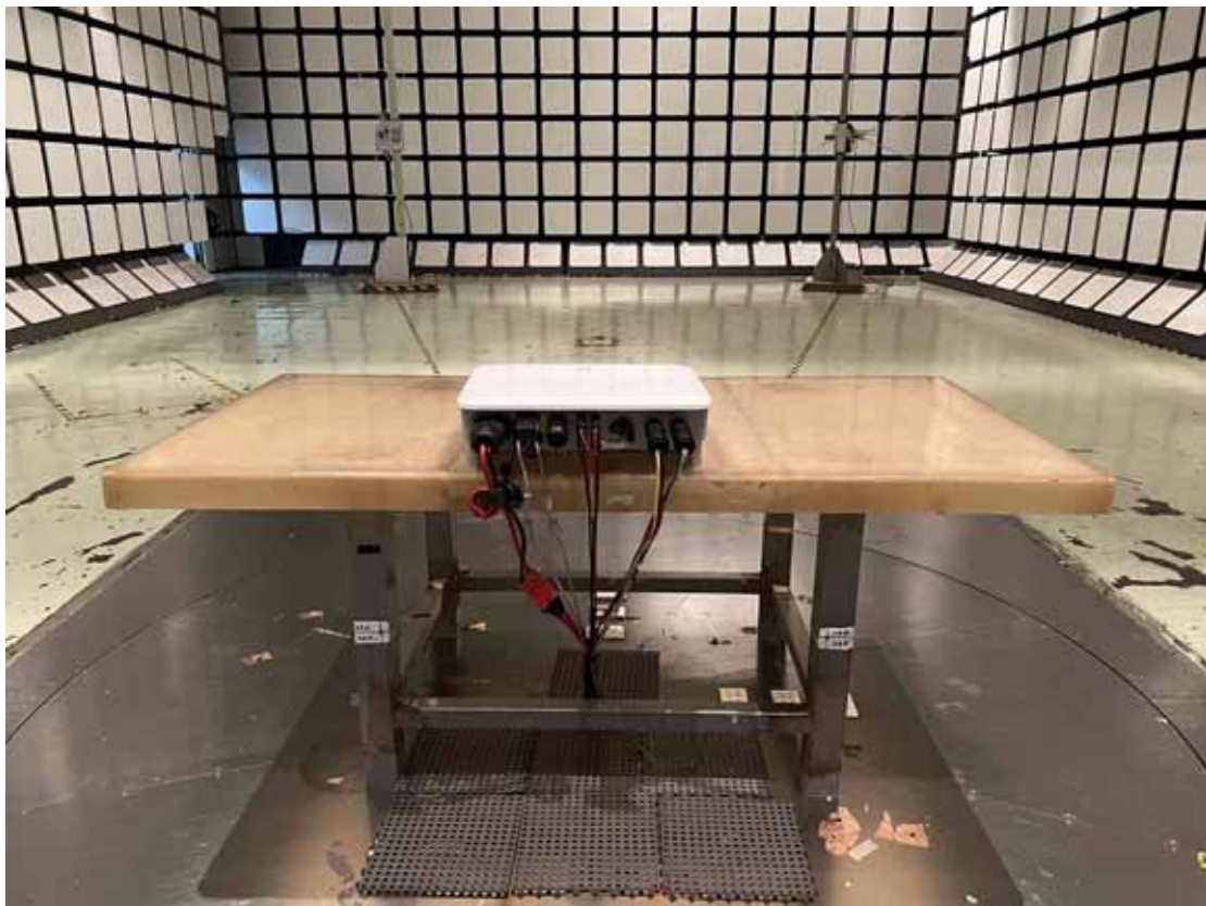
Back View of Radiated Disturbance Measurement
