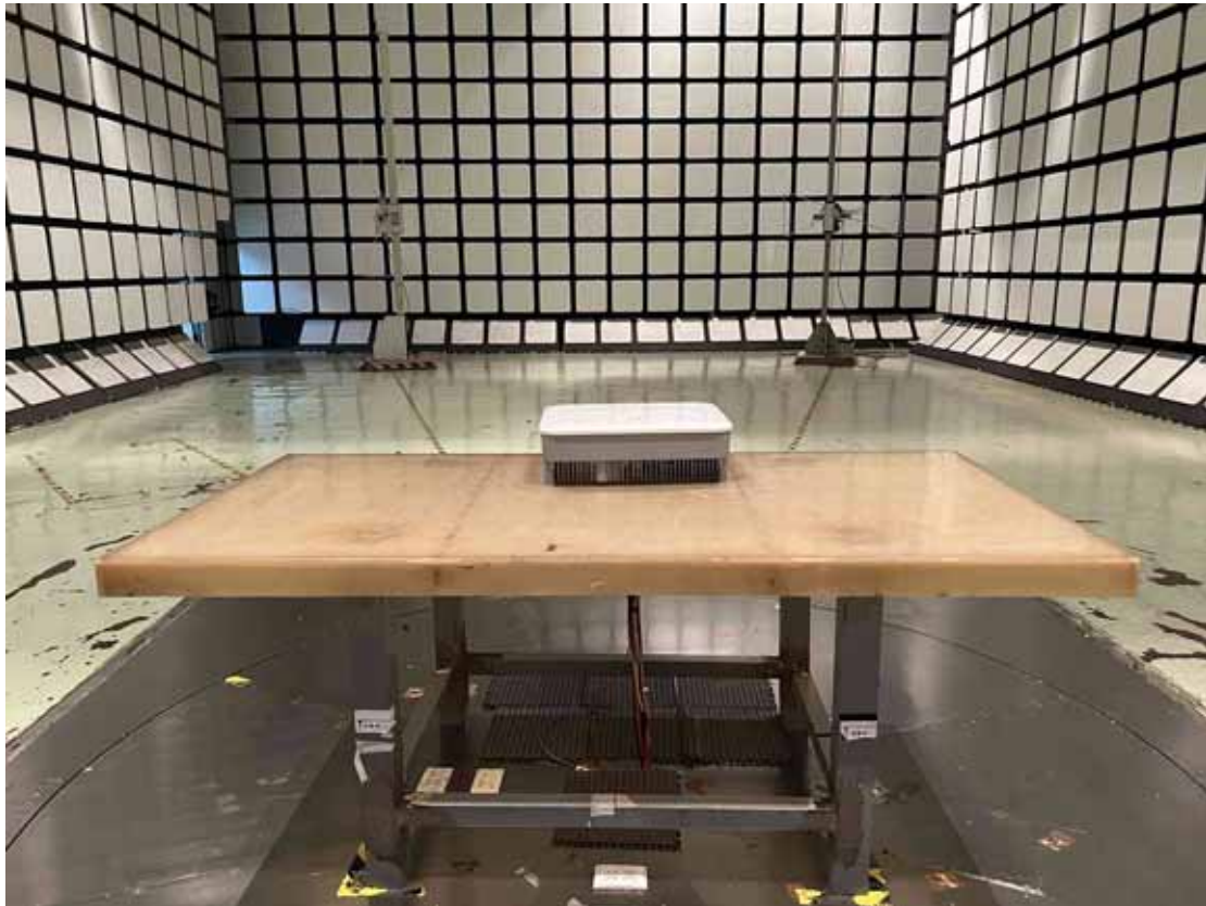
Front View of Radiated Disturbance Measurement
