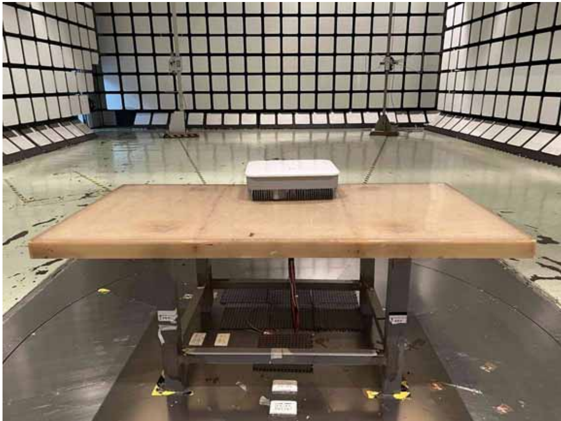
Front View of Radiated Disturbance Measurement
