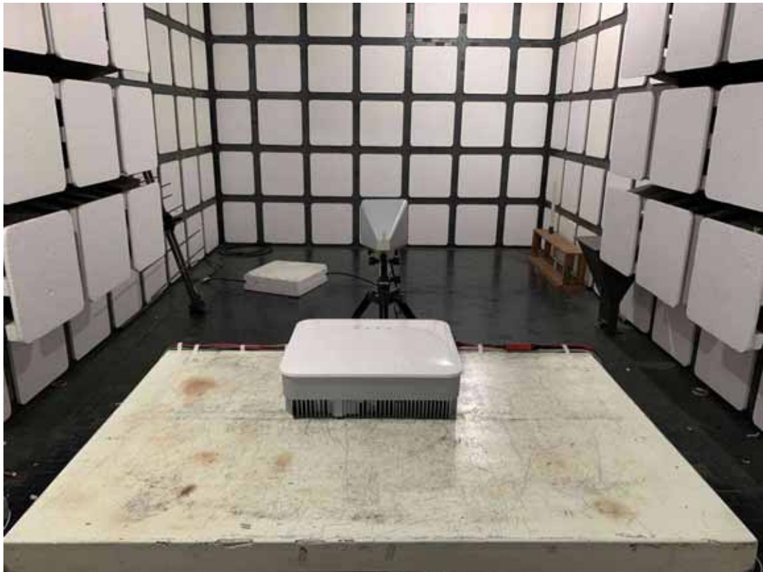
Front View of R/S Test (Above 1GHz)
