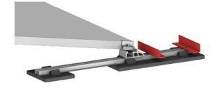
Use as much ballast as possible in front of the first row of each array per module and distribute the remaining ballast in the area of the back upstand. Position the building protection mats in accordance with the ballast centre of gravity.
