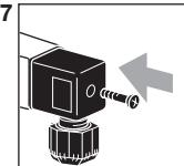
→ Pressure switch DG can be used in Zone 1 and 2 hazardous areas if an isolating amplifier is installed upstream in the safe area as “Ex-i” equipment pursuant to EN 60079-11 (VDE 0170-7):2007
