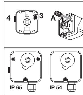
→ Use filter pad A, in the event that the electrical contacts in the DG may be soiled by dirt particles in the surrounding air/in the medium (Order No. 74916199; standard with IP 65).
