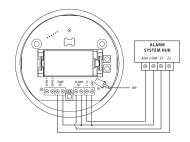
Figure 4.17: Connection with alarm system
