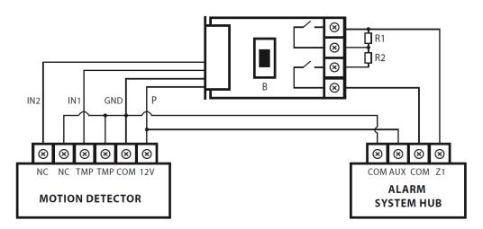
Figure 4.4: Universal Binary Sensor, parametric alarm line
