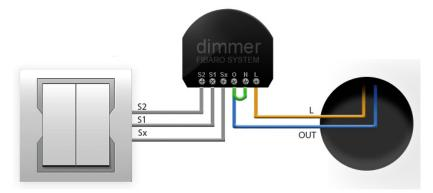
Figure 3.7: Dimmer wiring diagram
