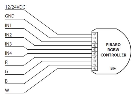
Figure 3.34: Fibaro RGBW Controller - Terminals description
