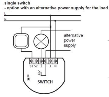
Figure 3.21: Single switch with an alternative power supply for the load
