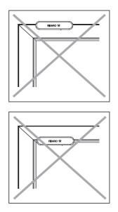
Figure 4.14: Door Window Sensor - incorrect sensor installation
