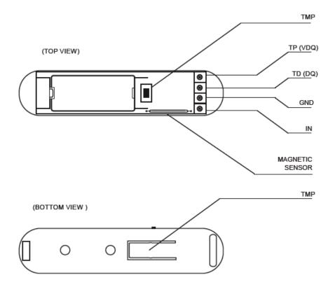
Figure 4.9: Door Window Sensor - general connections description
