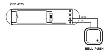
Figure 4.11: Door Window Sensor - example connection to momentary switch
