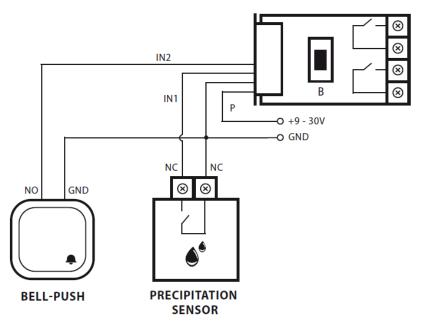
Figure 4.7: Universal Binary Sensor connection diagram
