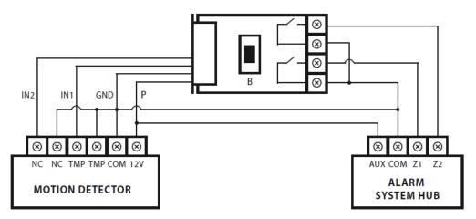
Figure 4.3: Universal Binary Sensor, standard alarm line
