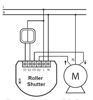
Figure 3.26: Wiring diagram - Roller Shutter
