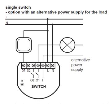
Figure 3.15: Single switch with an alternative power supply for the load
