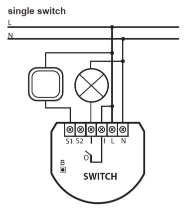
Figure 3.20: Single switch, Relay Switch 1x3kW wiring diagram
