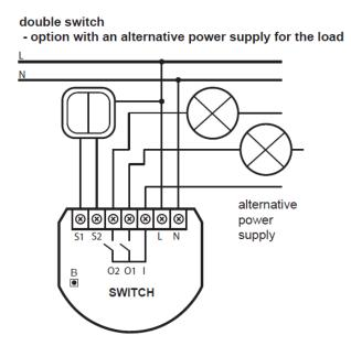
Figure 3.17: Double switch with an alternative power supply for the load
