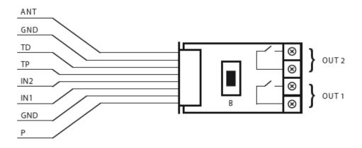
Figure 4.2: Universal Binary Sensor - connections description
