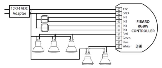
Figure 3.35: Fibaro RGBW Controller - Connecting halogen lighting
