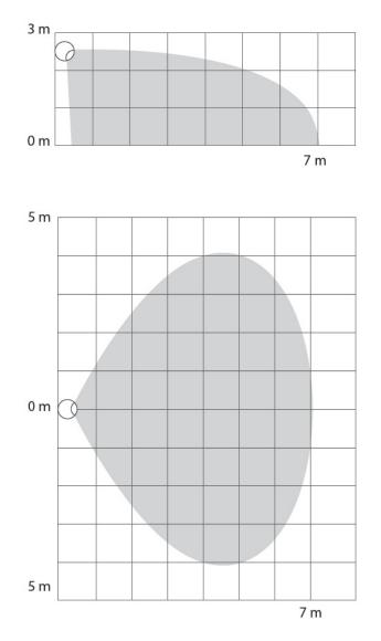
Figure 4.26: Fibaro Motion Sensors motion detection area
