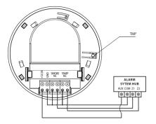
Figure 4.23: Alarm system hub connection
