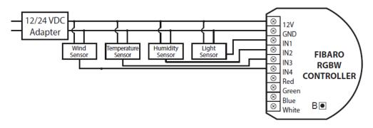
Figure 3.36: Fibaro RGBW Controller - 0-10 V sensors wiring diagram
