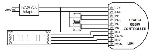
Figure 3.37: Fibaro RGBW Controller - RGBW strip wiring diagram
