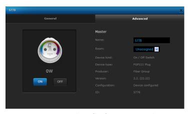
Figure 3.2: Plugs Configuration Window
