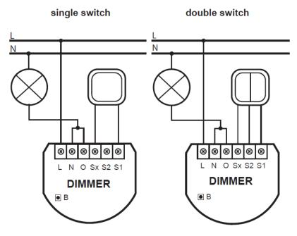
Figure 3.8: Dimmer wiring diagram - 2-wire connection
