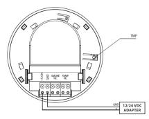
Figure 4.22: DC Power adapter connection
