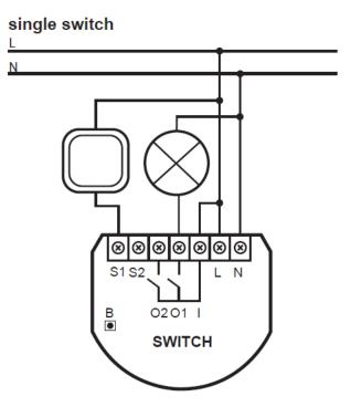
Figure 3.14: Single switch, Relay Switch 2x1,5kW connection diagram
