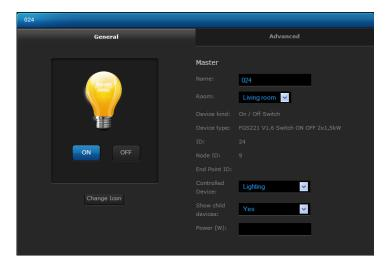
Figure 3.13: Relay Switch 2x1,5kW configuration window
