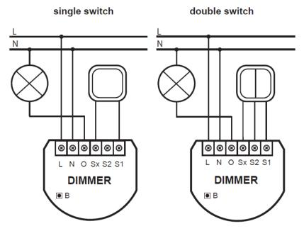
Figure 3.9: Dimmer wiring diagram - 3-wire connection
