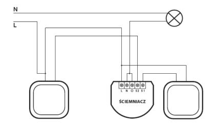
Figure 3.10: Dimmer wiring diagram - 3 way connection
