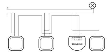
Figure 3.11: Dimmer wiring diagram - 4-way connection
