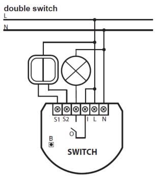
Figure 3.22: Double switch, Relay Switch 1x3kW wiring diagram
