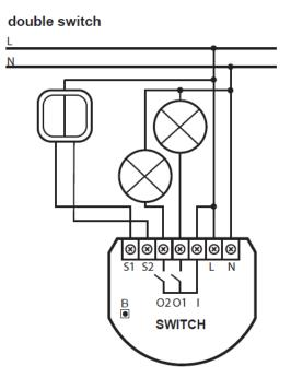
Figure 3.16: Double switch, Relay Switch 2x1,5kW connection diagram
