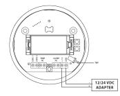
Figure 4.18: Connection to a constant power source
