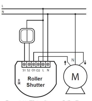
Figure 3.29: Wiring diagram - Roller Shutter
