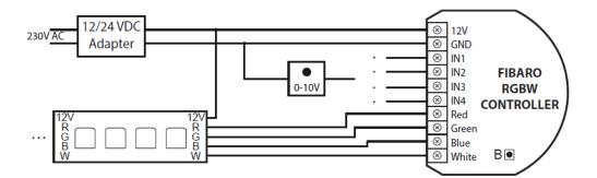
Figure 3.38: Fibaro RGBW Controller - RGBW strip 0-10V potentiometer wiring
