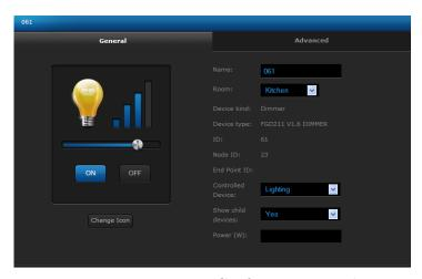
Figure 3.6: Dimmers Configuration Window
