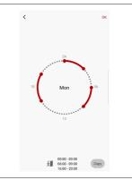
The Danfoss Ally™ App display shows both the 24 hour clock wheel, showing 'At Home' time in red and a summary of schedule, with the detailed times set. The minimum 'At Home' period is 30 minutes.
