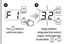
**NOTE:** Module starts to supply voltage at the output when any threshold is selected. The current value change causes a fan speed change - this allows you to check its operation and select adequate speed.
