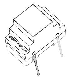
To open the casing of the module, you need to pry all the hooks (with a flat screwdriver) and then carefully remove its upper part.
