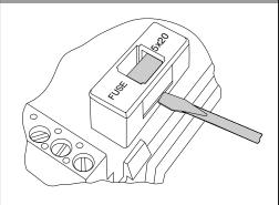
Using a flat screwdriver, pry the fuse holder, replace the fuse, put the holder back in place and then snap the upper housing of the module.
