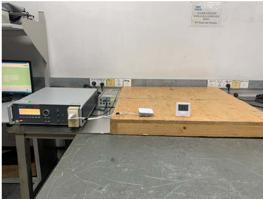
6.5. Photograph of set-up for Fast transient, common mode
