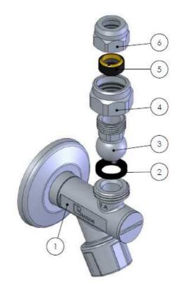
For a correct assembly of the undersink taps, please follow the above steps, checking carefully the assembly direction of the cartridge and the gaskets.
