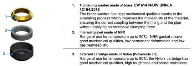
The RCC cartridge is the most safe and functional solution for the connection of taps to the final utilities. Being composed of three parts gathered in one single body, the RCC cartridge is the final solution to the installation problems of the compression fittings. No more parts lost or wrongly assembled, but one single piece which ensures an excellent mechanical and hydraulic tightness.
