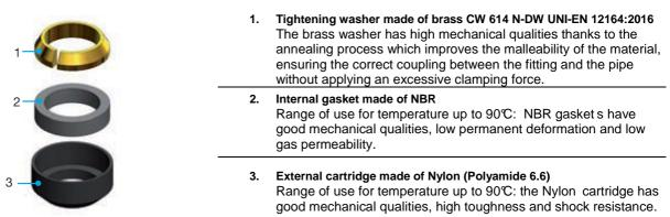
The RCC cartridge is the most safe and functional solution for the connection of the undersink taps to the final utilities. Being composed of three parts gathered in one single body, the RCC cartridge is the final solution to the installation problems of the compression fittings. No more parts lost or wrongly assembled, but one single piece which ensures an excellent mechanical and hydraulic tightness.
