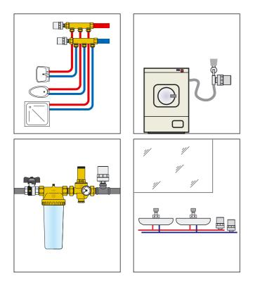
When installing the water hammer arrester under sinks and washhand basins, code 525130, create a space of 5-6 cm between the copper pipes and the threaded section of the shut-off valves. The radial connections enable water hammer arrester to be rotated to fit the available space.
