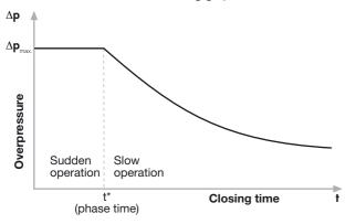
Numerical example: pipe length 10 m, diameter equivalent to 1/2", steel, copper and PE-X pipes with water velocity  $v_1 = 2$  m/s. We give the values of the velocity of the perturbation propagation  $v_2$ , sudden operating times t\* (phase time) and the overpressure  $\Delta p$  obtained with the formulas.
