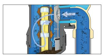
3. At the device outlet, the water passes through a filter mesh, which retains the residual impurities by mechanically selecting the particles according to their size. The large filter mesh surface with a mesh size of 160µm makes less prone to clogging.
