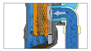
2. A central magnet captures and retains ferrous impurities down to the smallest sizes.
