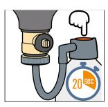
Additives can be injected using pressurised canisters.
