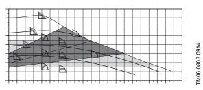
Fig. 21 UPM3 AUTO/HYBRID control modes with pump curves
