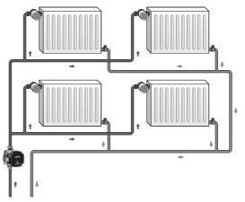
Fig. 3 Two-pipe heating system
