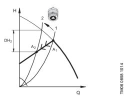
Fig. 24 Circulator operated in proportional-pressure control mode
