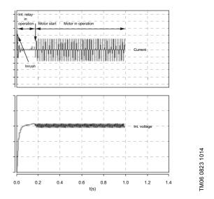
Fig. 56 Example: UPM3 with internal inrush relay
