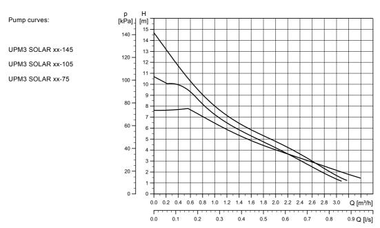
Fig. 10 Performance range UPM3 SOLAR, cast iron pump housing
