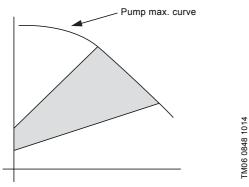
Fig. 26 Proportional pressure AUTO<sub>ADAPT</sub> operation area
