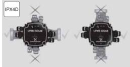
Fig. 49 Control box positions
