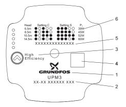
Fig. 6 Nameplate: Grundfos with setting indication
