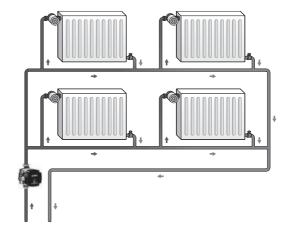
Fig. 2 One-pipe heating system
