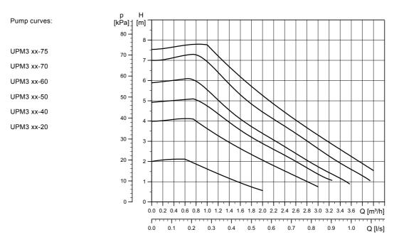
Fig. 9 Performance range UPM3, cast iron pump housing
