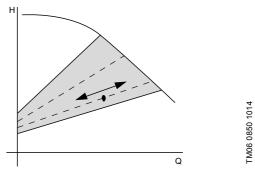
Fig. 30 New lower proportional pressure curve
