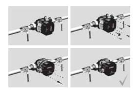
Fig. 50 Changing the control box position
