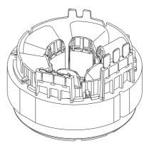
Fig. 34 Stator
