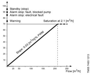
Fig. 16 PWM feedback signal - flow estimation
