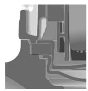
Fig. 44 Sectional drawing showing sealing principle of gasket
