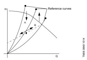
Fig. 29 Duty point on selected proportional pressure curve
