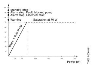
Fig. 15 PWM feedback signal - power consumption
