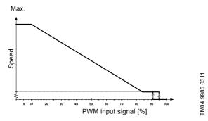
Fig. 13 PWM input profile A (heating)
