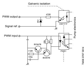
Fig. 12 Schematic drawing, interface
