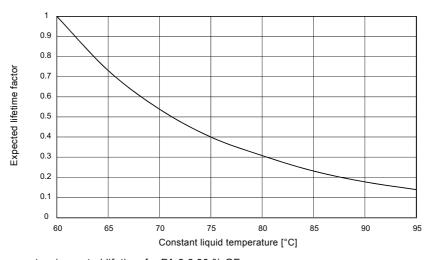
Fig. 47 Diagram temperature/expected lifetime for PA 6.6 30 % GF
