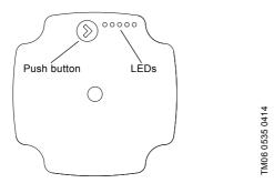
Fig. 17 User interface with one push button and five LEDs
