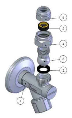
For a correct assembly of the undersink taps please follow the above steps, checking carefully the assembly direction of the cartridge and the gaskets.
