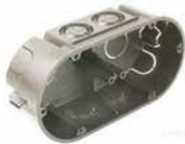
**UGD 2**, outlet box, flush type, twin gang; black (RAL 9005), for mounting of twin gang devices in standard distance of 71mm, mounting screw spacing 60mm
