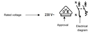
. The terminals upstream and downstream of the neutral pole are marked with an "N" moulded close to the screw heads.
