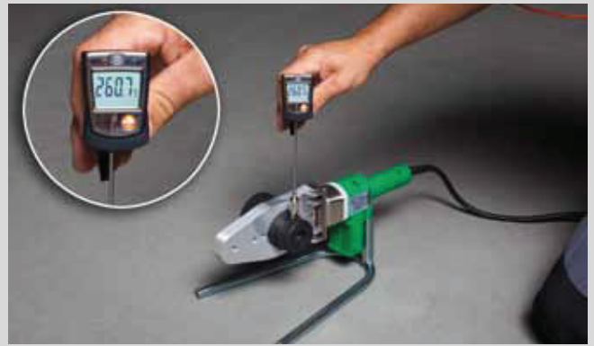
Measurement of temperature at the aquatherm manual welding device (800W )
