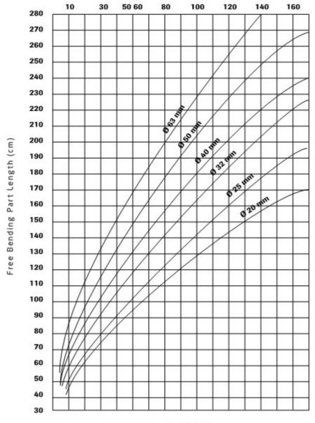
Lengthwise Stretching  $\Delta$  L (mm)
