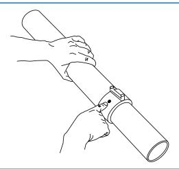
10) An incomplete welding can be verified by the fact that the indicator on the electrofusion sleeve has not changed colour (from white to black). Attention: the indicator does not guarantee a perfect weld which can be influenced by numerous factors such as dimensional tolerances, the ovality of the components to be welded, mechanical stress in the connection area. The parts to be welded must remain in position and aligned; they must not be subjected to any mechanical stress during cooling.
