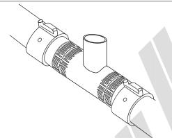
6) Position the piece of pipe or fitting in the space created between the two ends of the pipeline.
