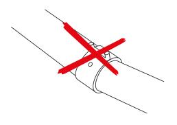
6) Keep the parts to be welded aligned and avoid any mechanical stress that could cause misalignment.
