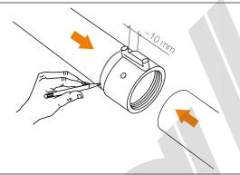
3) Clean and dry the welding ends. Mark a length of at least 10 mm greater that the insertion length of the electrofusion coupling on the pipe with a pencil, if necessary by temporarily inserting the parts into the coupler.
