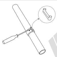
11) If required, the electrical connector sockets on the electrofusion couplings can be removed at the end of the cooling phase
