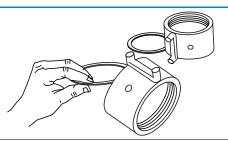
4) The electrofusion sleeves have a central ring that can be removed to turn the coupling into a sliding sleeve.
