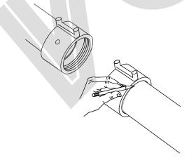
3) Insert the electrofusion sleeves onto each of the two ends and, when fully inserted, mark the insertion depth.
