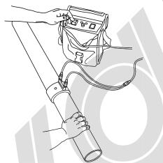
8) The welding time is determined automatically by the machine, which, when completed, will produce an audible signal. On no account can the same coupling be welded twice.
