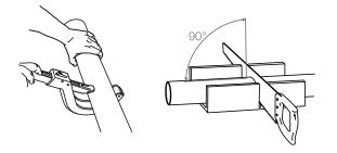
The pipes must be cut square so that the coils of the electric sleeve remain in contact with the pipe and/ or fitting.
