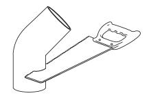
2) If necessary the ends of the fitting can be shortened as long as the remaining part is not shorter than the insertion depth of the electric sleeve as indicated on the technical card.
