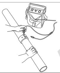
7) Connect the electrofusion sleeve to the welding machine using the appropriate plugs according to the diameter to be welded (for more information please see the welding machine handbook).
