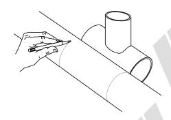
Indicate the area to be cut at a distance that is at least equal to the length of the electrofusion coupling or the fitting to be inserted in the pipe section.
