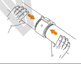
5) Inserts the parts to be welded into the sleeve coupling up to insertion depth. The connection with the sleeve must be free of tension such as those caused by any bracketing clips previously tightened near the weld area. The welding ends must remain dry during the whole welding process.
