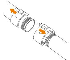
5) Position the electrofusion couplers in the space created between the two ends of the pipeline and slide them over the two ends.
