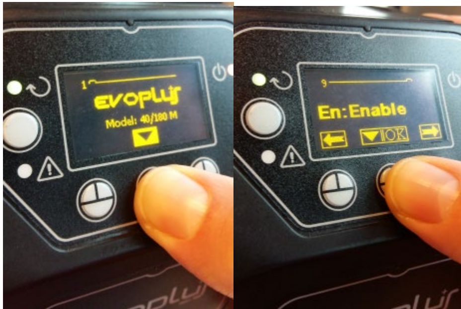
Figure 10- Software configuration of the multifunction module
