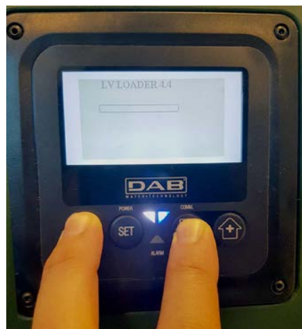
Figure 9C - Loader access for e.sybox
