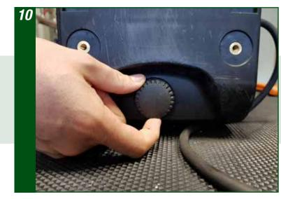
Unscrew the self-priming valve access cap
