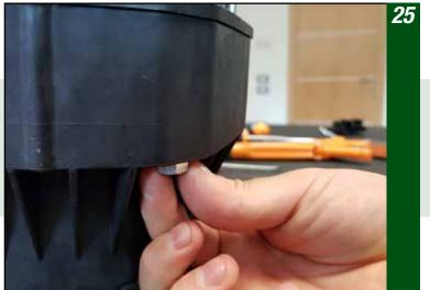
While screwing, keep the nut in position
