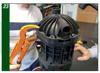
Using the two multi-grip pliers (and the rubber hammer if required), close the pump body
