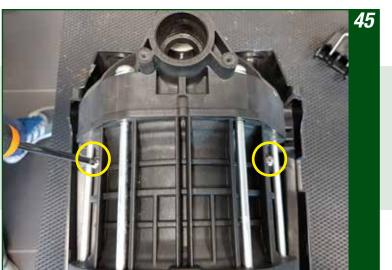
Then use the rubber hammer to detach the cover from the pump
