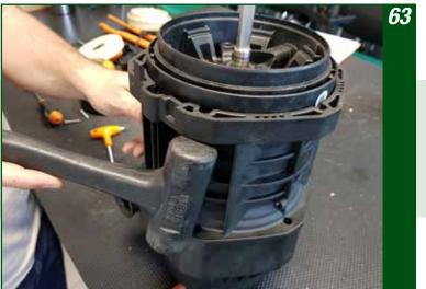
By means of the rubber hammer, remove the casing
