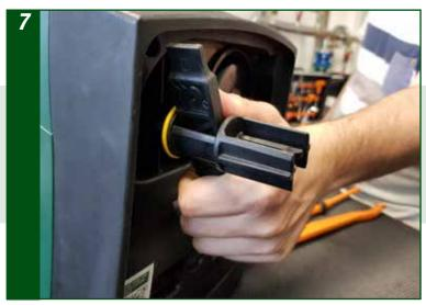
With the resulting composite tool, unscrew the all the external caps
