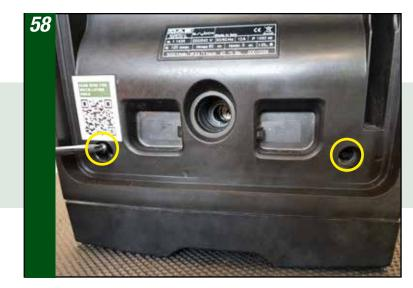
Screw the two screws highlighted in the picture
