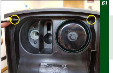
To fasten the front cover, screw the two screws seen in this picture, on the top-cover side, and the two in the following picture, on the bottom-cover side
