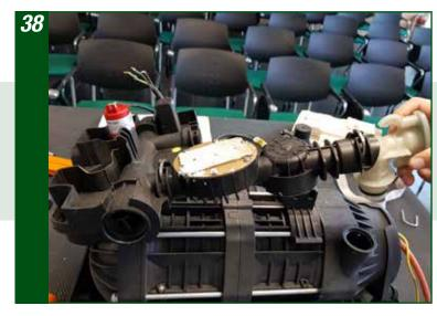
Lift and remove the sensors block
