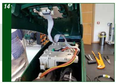
Lift the front cover, paying attention not to pull the flat cable excessively
