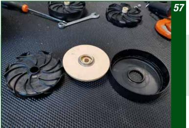
If required, dismantle the stages in their single parts: diffuser (conveyor, left, and diffuser box, right) and impeller (middle)
