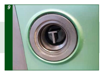
Pull out the non-return valve. Use the composite tool (or pliers)
