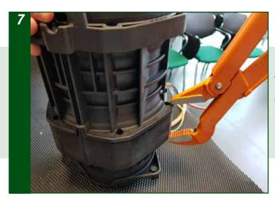
Using the two multi-grip pliers, tighten the two parts, acting on opposite sides at the same time (be careful not to damage the plastic)
