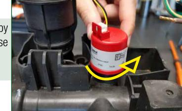
Remove the pressure sensor by unscrewing it counterclockwise
