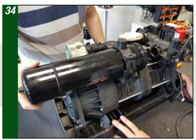
Insert the pressure vessel through its support and into its fitting
