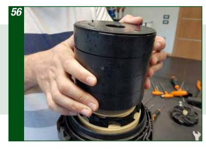
You should be able to remove the other stages (or most of them) all together, otherwise keep using the screwdrivers to facilitate the operation
