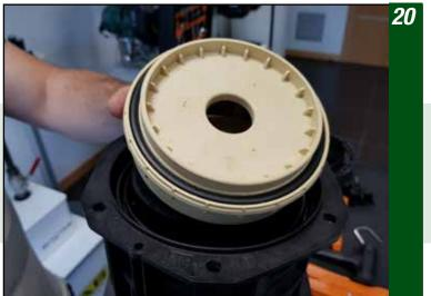
Install the pump body's O-ring
