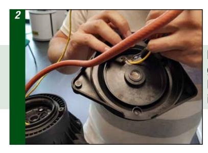
Insert the motor cable and the ground wire in the hole of the lower motor cover, and let it slip in position
