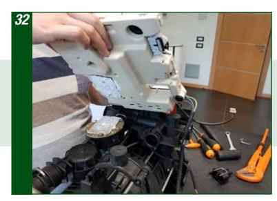
Gently lift and remove the main board block
