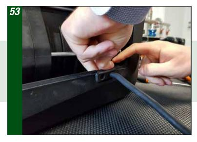
Before inserting the left-side cover, place the cable gland in the right position
