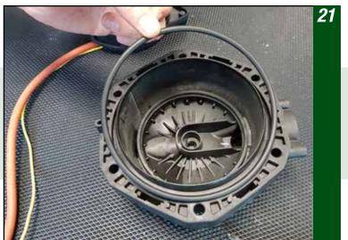
Insert the pump body in the right position (see picture)
