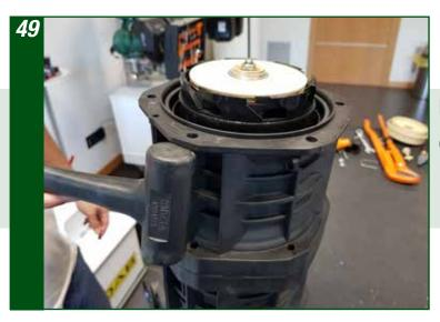
Use the rubber hammer to detach the outer cover
