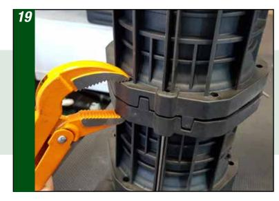
By means of the two multi-grip pliers, tighten the body downwards, acting on opposite sides at the same time (be careful not to damage the plastic)
