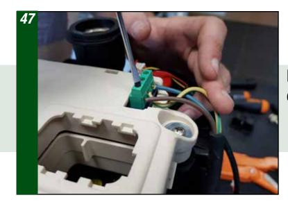
Insert and fasten the power cable wires
