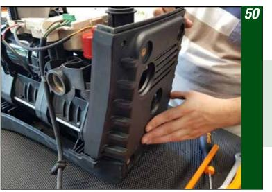
Screw the four screws highlighted in this picture and in the following one
