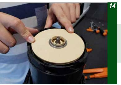
Always push downwards to make sure all the hydraulic parts are well packed
