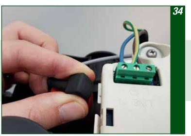
Before removing the pressure sensor, remove the protection cap to check the state of the connection wires
