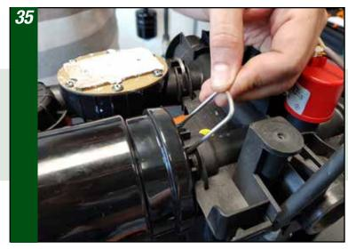
Secure the vessel by inserting the klammer
