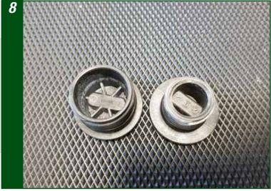
Note that the non-return valve access cap (left) has a bigger size than the other ones (1 ¼" vs 1"). Be careful not to mix them up when reassembling the pump
