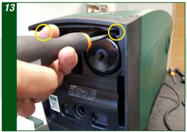
To remove the front cover, unscrew the highlighted screws from the top cover and the bottom cover
