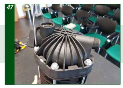
Unscrew the six torx screws (T40 torx screwdriver) and use the rubber hammer to remove the pump body
