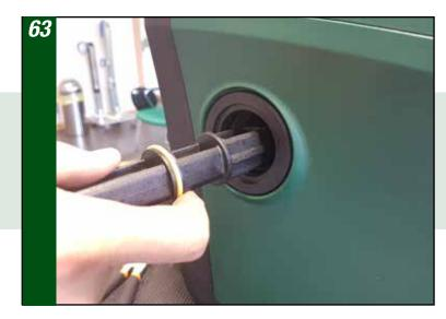
Use the composite tool to insert the non-return valve
