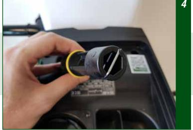
The small key may be used to unscrew the front display's small screws. This will allow the user to rotate the display and adapt the view to the position of installation
