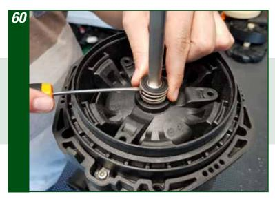
Remove the mechanical seal's rotating part
