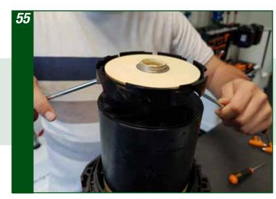
Using two screwdrivers as levers, lift and remove the first stage
