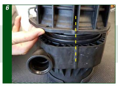
Insert the main motor casing, aligning the parts as shown in picture
