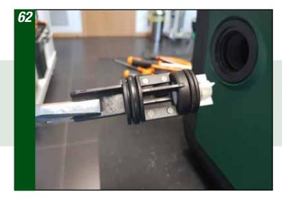
Before reinstalling the non-return valve, check/replace the O-rings
