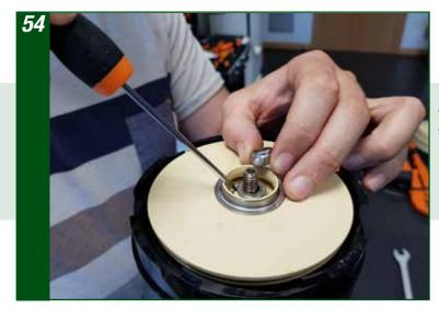
After removing the nut, remove the washer
