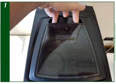
Pull up and remove the transparent cover
