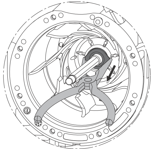
Fig. 12 Removing the stationary shaft seal
