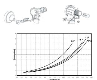
Application: Patented hydraulic regulator that eliminates the classic defects of such devices. Especially suitable for filling storage tanks or cisterns.
