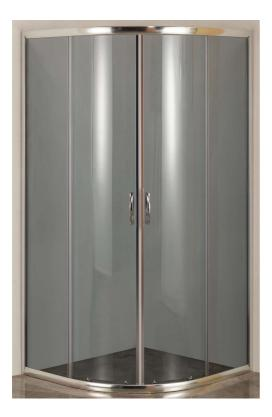
Code: Type: Generic size: Adjustment: Height: Profiles: Glass thickness (mm): Glass type: Shower tray: Handle: Hinges: SW-815S Chrome Shower enclosure 900\*900 mm 885-890 mm 1800 mm Aluminum frame in chrome 4 Tempered grey glass Not included Chrome plastic Zinc and plastic, chrome Up - double rollers Down – single rollers R55
