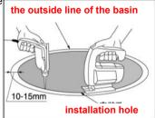
3.Installing tap and drainer on wash basin according to the installation requirment and steps
