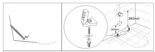
Position pan against wall and mark off pan fixing holes on floor.
