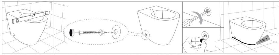
Ensure that pan is level. Fix pan to floor using fixing screws and flexible sealant. Install soft closing seat.
