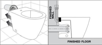
Push pan back into position. Ensure that you make a firm connection wilh inlel and outlet pipes and avoid distu disturbing the floor fixing brackets. Flush test for leaks.
