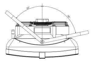
Use flexible connections to allow the heater to be turned to the sides. Depending on the flexible connections, the maximum turn is 78° to both sides. Figure shows maximum angle to one side and 50° to the other with minimal distance left for connections.
