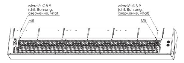
Drawing below shows the position of the mounting holes for the pins
