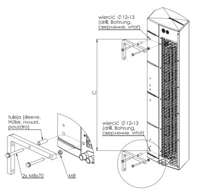
It is important to note that the minimum distance between the unit and the floor for installation with engine at the bottom is not less than 100mm. This allows access to the electrical terminal strip and to the water exchanger vent.
