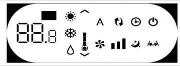
Normally, the display shows the operating status (see Description of machine functioning paragraph) as well as any alarms (see Display alarms paragraph). In addition, it is possible to select the various functions by pressing the symbols.
