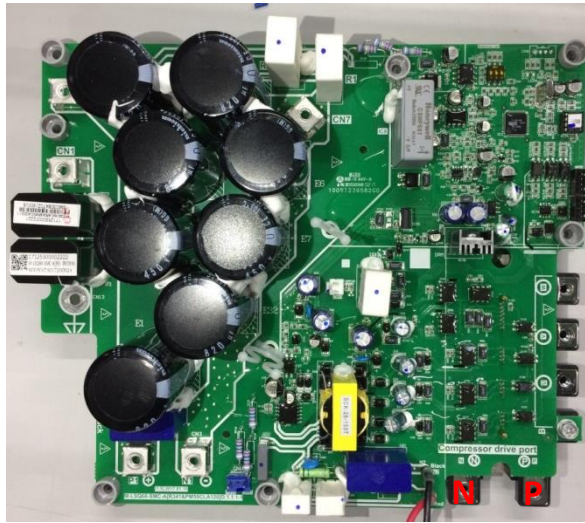
Figure 4-4.9: Inverter module terminals
