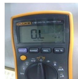
Figure 4-4.5: Measuring resistances between compressor terminals and ground
