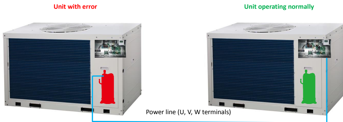
Figure 4-4.11: Connecting compressor to an error-free unit
