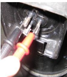
Figure 4-4.4: Measuring resistances among compressor terminals
