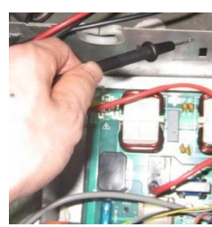
Figure 4-4.5: Measuring resistances between compressor terminals and ground
