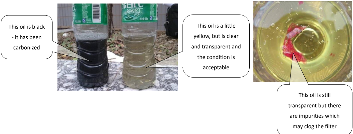
Figure 4-4.13: Inspecting compressor oil
