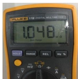
Figure 4-4.4: Measuring resistances among compressor terminals
