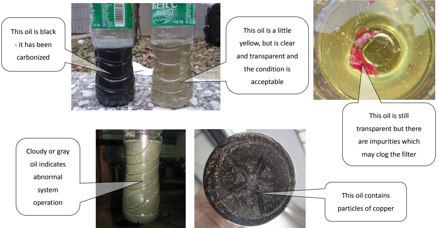
Figure 6-2.10: Inspecting compressor oil
