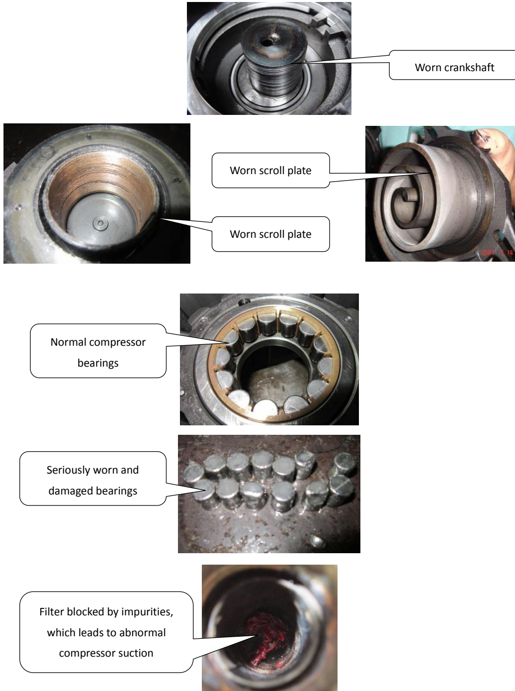
Figure 6-2.11: Effects of spoiled compressor oil
