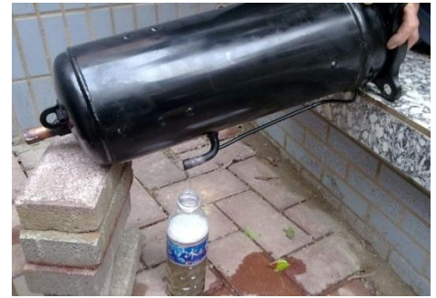
Figure 6-2.8: Draining oil from a compressor
