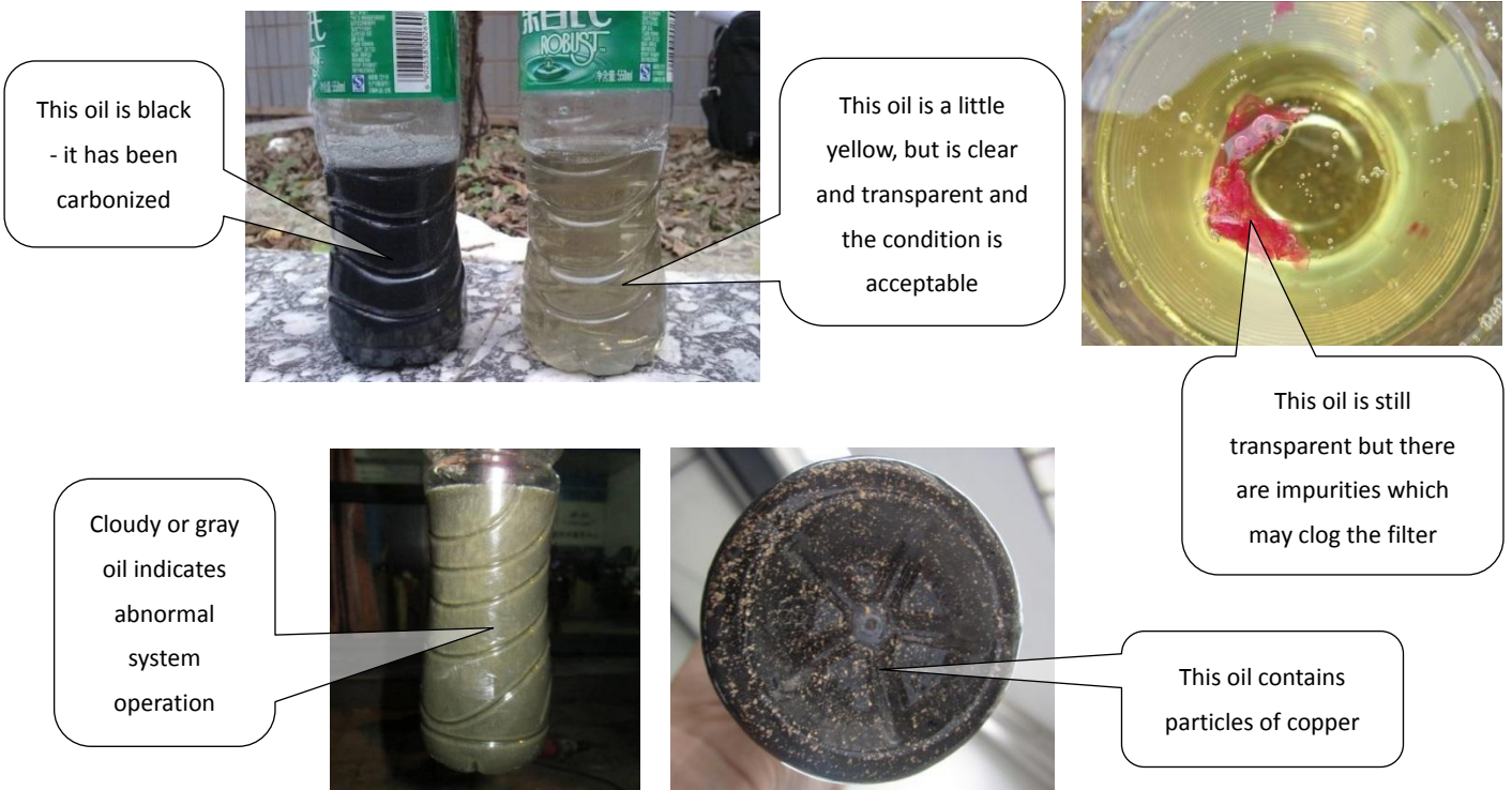
Figure 6-2.10: Inspecting compressor oil
