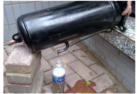
Figure 6-2.8: Draining oil from a compressor
