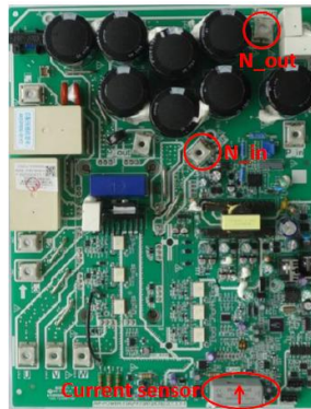
Figure 6-2.2: DC detection wire connection method
