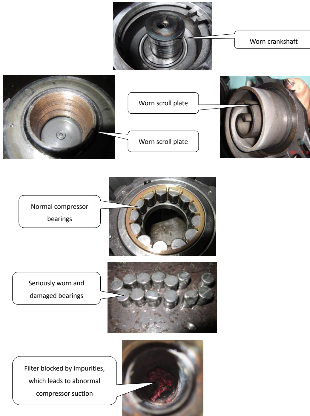
Figure 6-2.11: Effects of spoiled compressor oil
