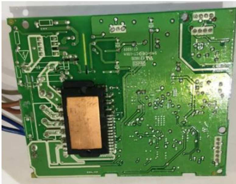
Filter board PCB for MV6-xyzWV2GN1-E and MV6-ixyzWV2GN1-E (xyz=, 400, 450, 500, 560, 615)
