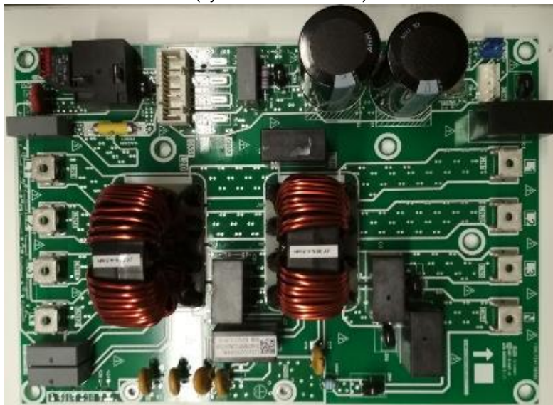
Filter board PCB for MV6-xyzWV2GN1-E and MV6-ixyzWV2GN1-E (xyz=252、280、335)
