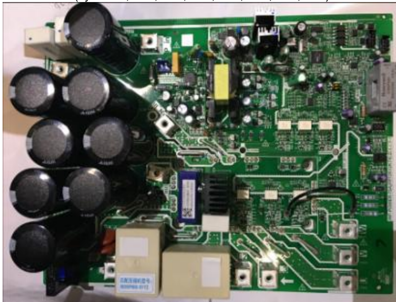
Inverter module PCB for MV6-xyzWV2GN1-E and MV6-ixyzWV2GN1-E (xyz=252, 280, 335, 400, 450, 500, 560, 615)
