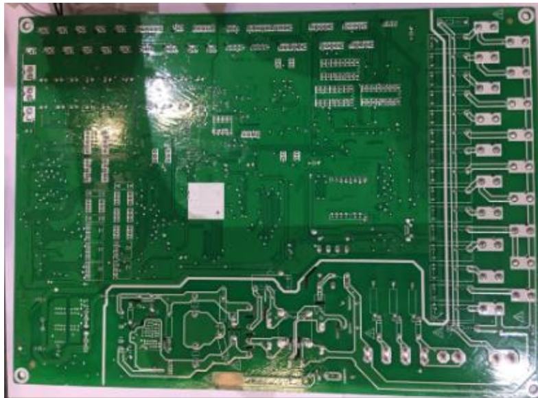
Inverter module PCB for MV6-xyzWV2GN1-E and MV6-ixyzWV2GN1-E (xyz=252, 280, 335, 400, 450, 500, 560, 615)
