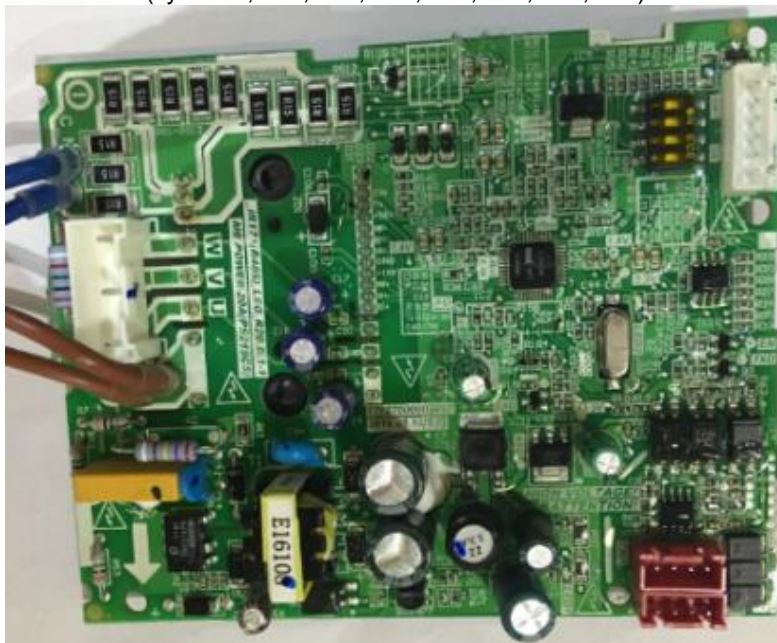
Fan driver module PCB for MV6-xyzWV2GN1-E and MV6-ixyzWV2GN1-E (xyz=252, 280, 335, 400, 450, 500, 560, 615)
