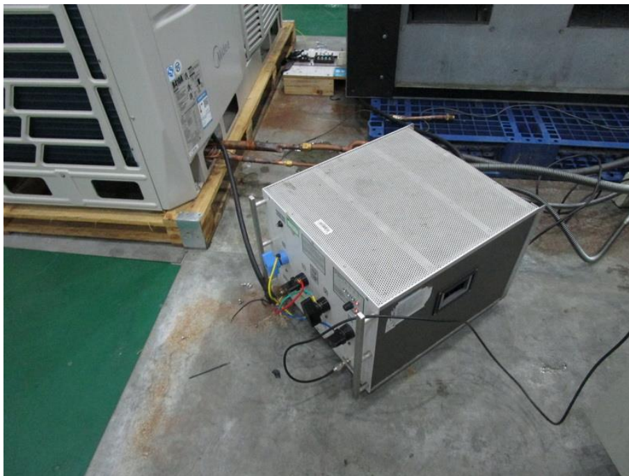
Photograph of Test Setup: Conducted Emissions 150kHz-30MHz
