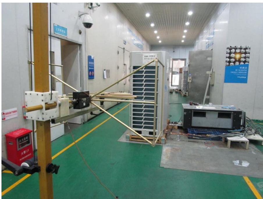
Photograph of Test Setup: Radiated Emissions 30MHz-1000MHz
