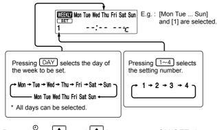
(3) Press  $\left[\frac{1}{(NV/OFF)}\right]$ ,  $\left[\frac{1}{M_{e}}\right]$ , and  $\left[\frac{1}{M_{e}}\right]$  buttons to set ON/OFF, time, and temperature.
