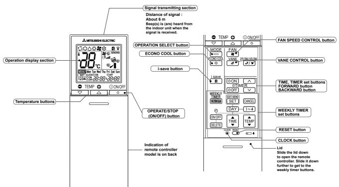
**NOTE**: Last setting will be stored after the unit is turned OFF with the remote controller. Indoor unit receive the signal of the remote controller with beeps.
