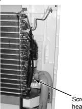
Screw of the heat exchanger
