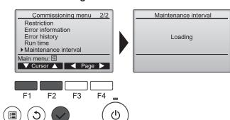
Press the  $\boxed{\texttt{F1}}$  and  $\boxed{\texttt{F2}}$  button to move the cursor. Press the  $\boxed{\checkmark}$  button to go to the next screen.
