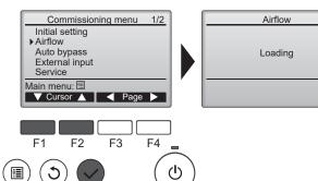
Press the  $\boxed{\texttt{F1}}$  and  $\boxed{\texttt{F2}}$  button to move the cursor. Press the  $\boxed{\checkmark}$  button to go to the next screen.
