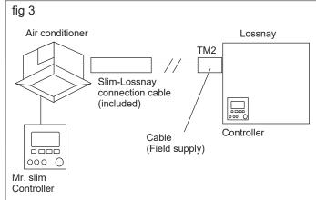
You can control the product by Mr.Slim's remote controller. Extend the Slim-Lossnay interlocking cable connected to Slim. Please attach to TM2 of the product.
