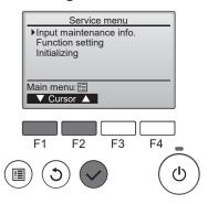
Press the  $\boxed{\texttt{F1}}$  and  $\boxed{\texttt{F2}}$  button to move the cursor. Press the  $\boxed{\checkmark}$  button to go to the next screen.
