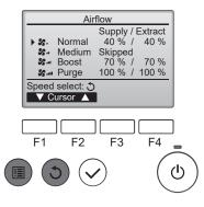
Press the (5) button to return to 6.4.3.2 Fan speed selection.
