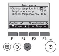
Press the  $\boxed{\texttt{F1}}$  and  $\boxed{\texttt{F2}}$  button to move the cursor. Press the  $\boxed{\texttt{F3}}$  and  $\boxed{\texttt{F4}}$  button to change the setting value. Press the  $\boxed{\checkmark}$  button to save the changes.
