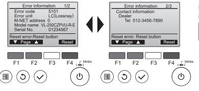
Press the F1 and F2 button to change the page. Press the F4 button to move to the Reset screen.
