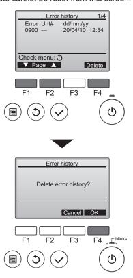
Press the F1 and F2 button to change the page. Up to 4 pages, 12 cases can be stored in the error history. Press the F4 button to move to the Reset screen.
