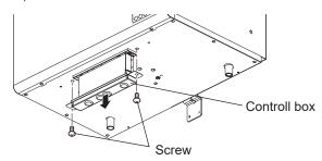
2) Remove an insulating sheet. (Be careful of the protrusions on both sides of the control box)
