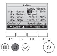
Press the ③ button to return to 6.4.3.2 Fan speed selection. Select other fan speed at 6.4.3.2.
