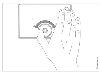
The scroll wheel comprises a sensor that is touch-sensitive. There is one key array each to the left and right of the scroll wheel. All required appliance functions are controlled and checked with the scroll wheel and the keys.
