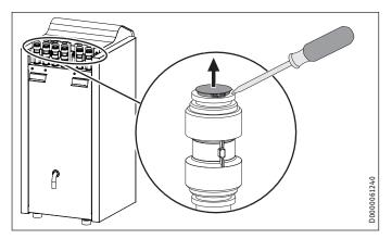
Remove the protective grey caps from the push-fit connectors.
