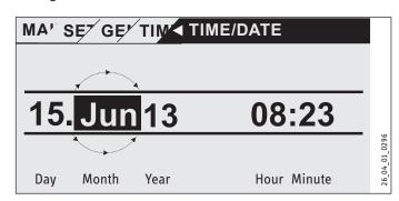
On activation, the highlighter is over the position MONTH. Confirm with OK. Set the current month with the scroll wheel and confirm with OK. A calendar page is displayed. Move the highlighter to the required day with the scroll wheel and confirm with OK. The new value is saved when you confirm with OK. Set the year, hours and minutes the same way.
