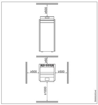
► Maintain the minimum clearances to ensure trouble-free operation of the appliance and facilitate maintenance work.
