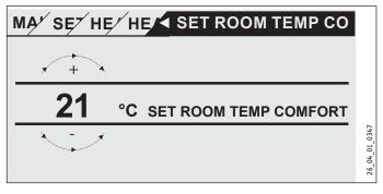
To enter set temperatures, a number surrounded by a circle appears on the display. This indicates that you can change the value by turning the scroll wheel.
