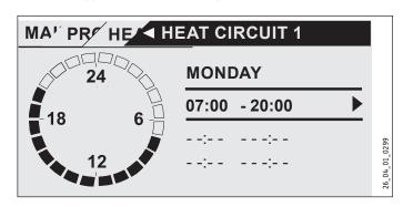
In this example, only one switching times pair has so far been programmed. For switching times pairs 2 and 3, you can see short dashes instead of times. These switching time pairs are still empty. If you select one of the free switching time pairs with OK, you reach the area where you can set the associated start and end times. Press OK and the display shown below appears. Set the required time with the scroll wheel.
