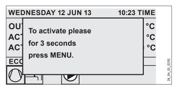
Touch the MENU key for three seconds to enable the programming unit.
