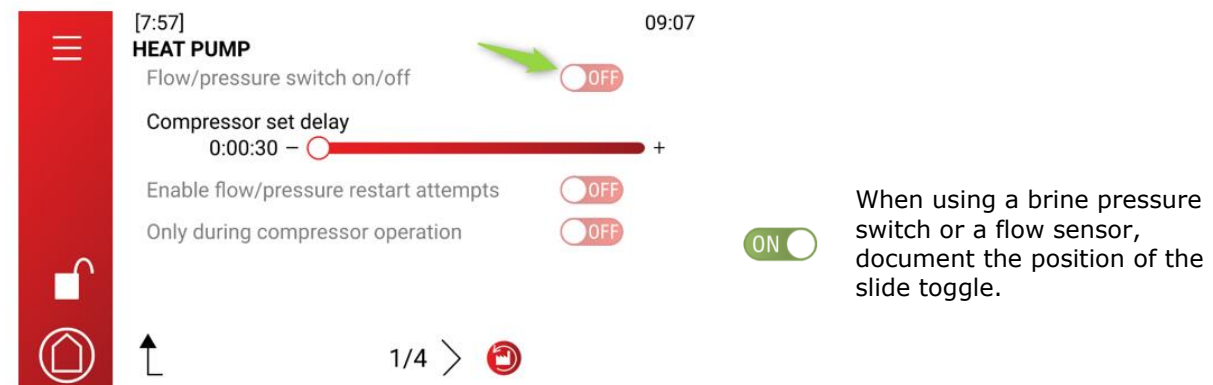
Figure 42 Heat pump-2 settings
