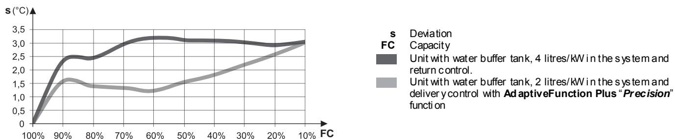
The chart shows the deviation of the water temperature from the set-point at various operating capacities, showing how a unit with delivery control and **AdaptiveFunction Plus "Precision"** function ensures greater precision in delivery water temperature.
