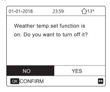
Move to "NO",press "OK" to come back to home page,move to "YES",press "OK" to reset the WEATHER TEMP\_SET
