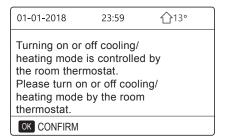
② The room thermostat is SET DOUBLE ZONE(see "ROOM THERMOSTAT SETTING" in "Installation and owner's manual "). The room thermostat for fan coil is turned off, the room thermostat for the floor heating is turned on, and the unit is running, but the display is OFF. The following page is displayed:
