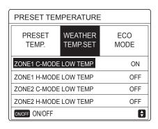
If the weather TEMP.SET is actived, the desired temperature can not be adjusted on the interface. Press the "▼"、"▲" to adjust the temperature on home page. The following page will appear:
