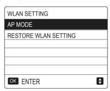
Activate the WLAN by interface. Go to "MENU"> "WLAN SETTING"> "AP MODE".
