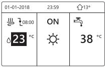
1) When the cursor is on the temperature of space operation mode side (Including heat mode -X, , cool mode \* and auto mode A), press "ON/OFF" key to turn on/off space heating or cooling.
