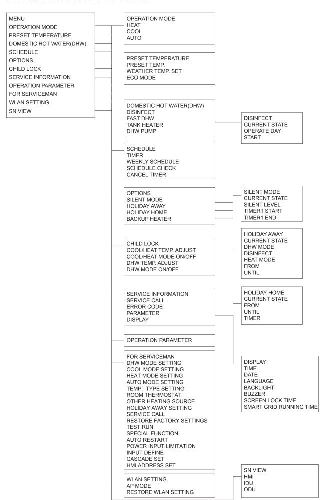
FOR SERVICEMAN 1 DHW MODE SETTING 2 COOL MODE SETTING 3 HEAT MODE SETTING 4 AUTO MODE SETTING 5 TEMP. TYPE SETTING 6 ROOM THERMOSTAT 7 OTHER HEATING SOURECE 8 HOLIDAY AWAY SETTING 9 SERVICE CALL 10 RESTORE FACTORY SETTINGS 11TEST RUN 12 SPECIAL FUNCTION 13 AUTO RESTART 14 POWER INPUT LIMI TATION 15 INPUT DEFINE 16 CASCADE SET 17 HMI ADDRESS SET
