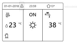
Press any key, the icon 🛈 will flash. Long press the "UNLOCK" key. The icon 🛈 will disappear, the interface can be controlled.
