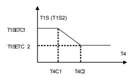
State: In the setting the wired controller, if T4C2<T4C1, then exchange their value; if T1SETC1<T1SETC2, then exchange their value.
